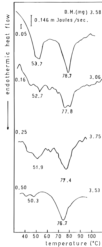
Figure 6. DSC thermograms of whole smooth muscle of scallop at different ionic strength values (pH 7.0). Heating rate = 10\text{ }^{\circ}\text{C}/\text{min} . DM, dry matter
